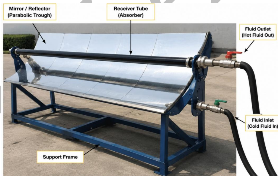
PTSC Prototype showing Mirror/Reflector, Receiver Tube, Fluid Inlet/Outlet and Support Frame.
